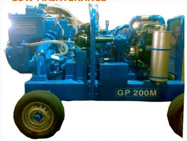
Another robust pump in the Oasis Sykes stable, the GP200 shares the same engineering pedigree and high efficiency priming system as all Oasis Sykes pumps. GP200 is used extensively on construction sites for dewatering, by oil companies, municipalities and utilities, and for marine applications.
